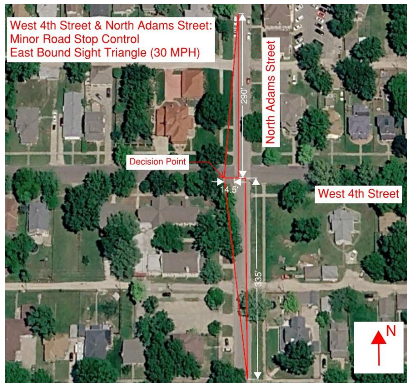
4 th & Adams - Two-Way Stop Control Eastbound Sight Distance
