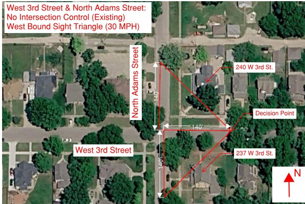
3 rd & Adams - No Intersection Control Westbound Sight Distance
