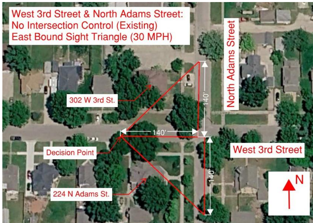
3 rd & Adams - No Intersection Control Eastbound Sight Distance
