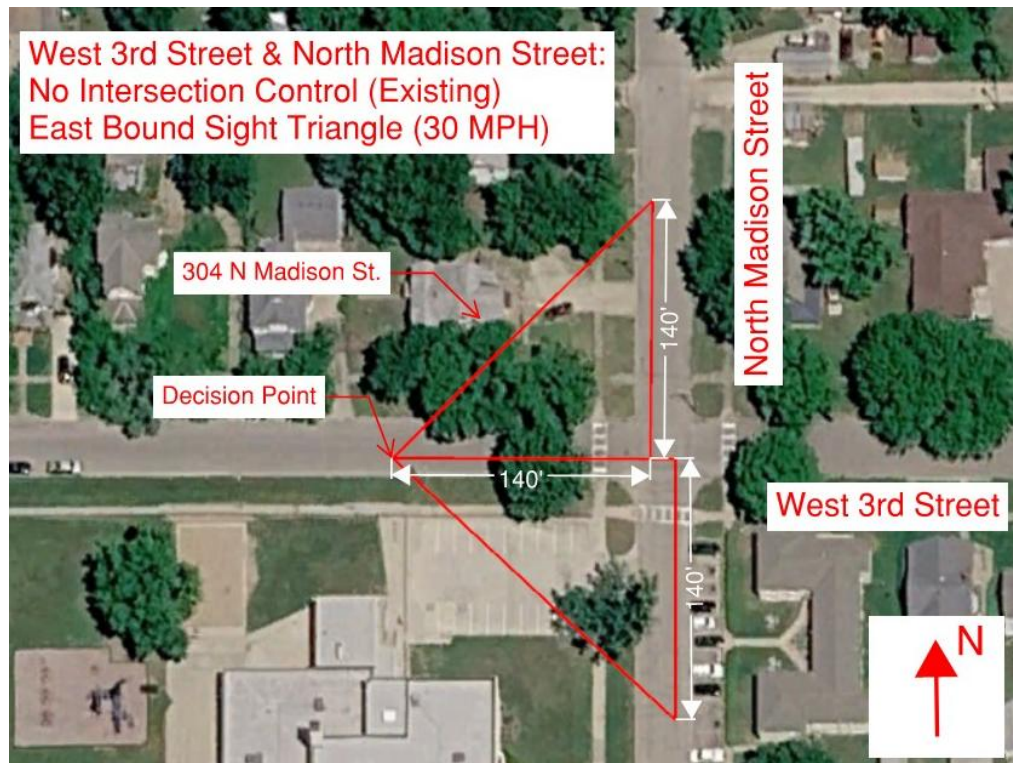
3 rd & Madison - No Intersection Control Eastbound Sight Distance
