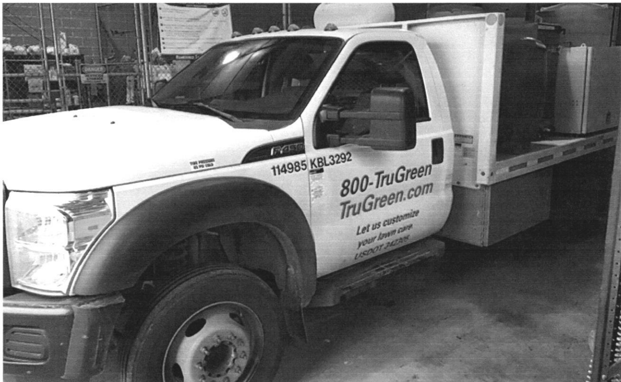
Ford F450 Spray Trucks (three) – two 200-gallon tanks and a 300-gallon tank
