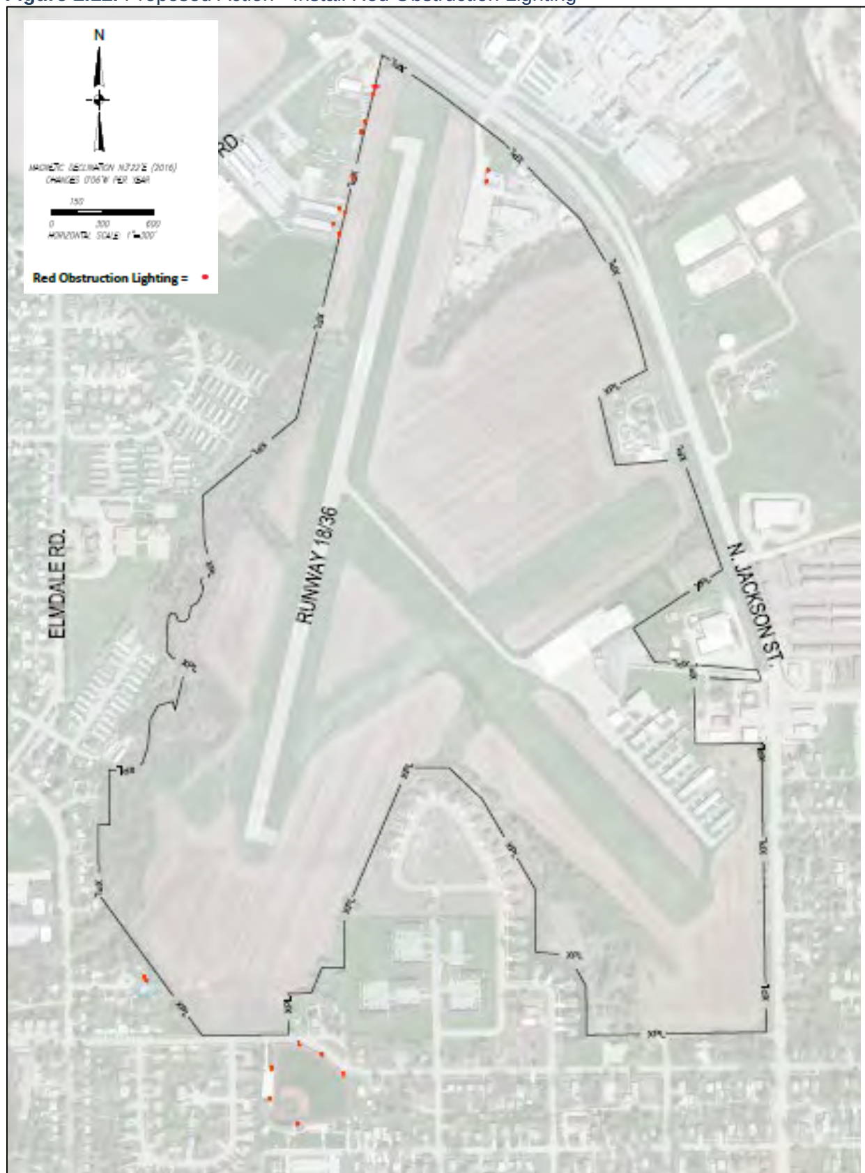
Figure 2.12. Proposed Action - Install Red Obstruction Lighting
